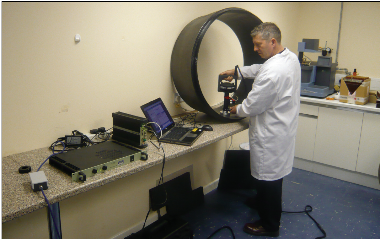
Fig. 1 Zero-splice, composite double-layer acoustic panel – QA test using Portable Impedance Meter Type 9737
