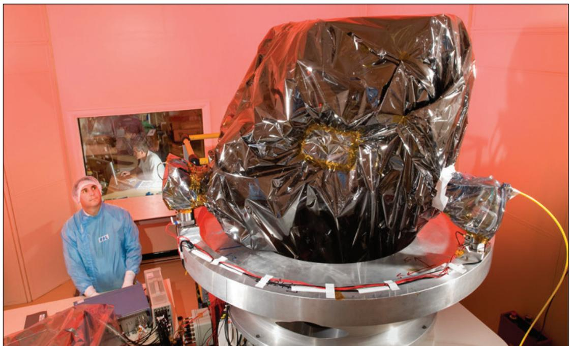
*RAL Space's V8 Shaker with MIRI Structural Model mounted on the guided load support platform*
