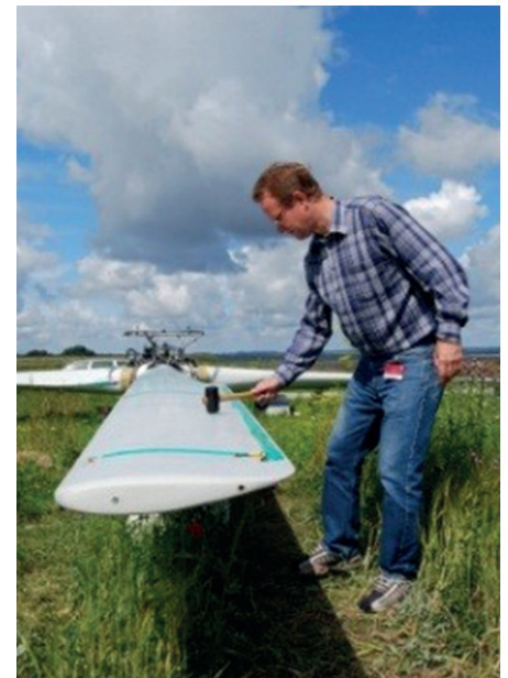
An OMA test using a rubber mallet was performed to check the system and the accelerometer mounting before the blade is reinstalled for a six-month test
