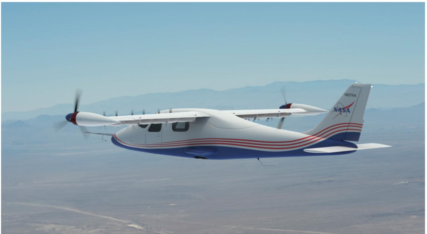
*Graphic Illustration of NASA's X-57 Maxwell in Mod 4 Configuration (12 High-Lift Motors and 2 Wingtip Cruise Motors)*
