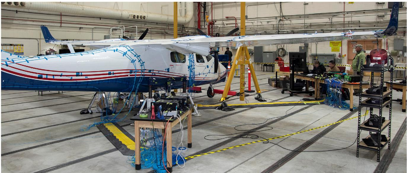
Overview of GVT setup on the X-57 Maxwell Mod II Configuration
