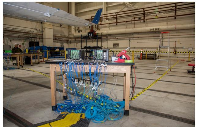
LAN-XI Mainframe #3 & #4 (two 5-slot mainframes)
