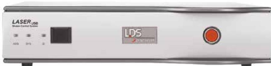
LASER<sub>USB</sub> has a USB 2.0 interface for easy PC connectivity, while its multiple DSP processors handle the control loop independently of the PC host.
