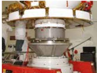
The Lin-E-Air shaker suspension system gives excellent isolation, reducing the the shaker's affect on the surrounding environment. An optional guided head expander ensures that loads with off-centre centres of gravity can be tested effectively and safely. The addition of a slip table enables products to be tested in both vertical and horizontal axes. The slip table is also available with a thermal barrier for use in environmental tests.
