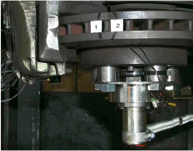
Figure 9. Location of accelerometers in the disc: 1 - Out-of-plane direction, 2 - In-plane direction. Note the slipring connector for transfer of the signals in the lower part of the picture.
