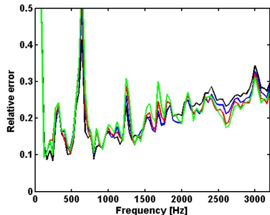
Figure 2: Relative difference between measured and calculated sound pressure for the four array distances. Black curve: 0.5 cm; blue curve: 1.5 cm; red curve: 3.0 cm; and green curve: 4.5 cm. The calculated sound pressures are based on measured velocities.
