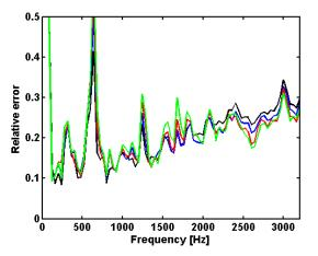
Figure 2: Relative difference between measured and calculated sound pressure for the four array distances.Black curve: 0.5 cm; blue curve: 1.5 cm; red curve: 3.0 cm; and green curve: 4.5 cm. The calculated sound pressures are based on measured velocities.
