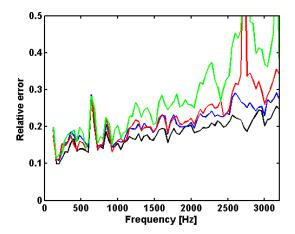
Figure 3: Relative difference between measured and calculated velocity for the four array distances using SONAH and NCP. Black curve: 0.5 cm; blue curve: 1.5 cm; red curve: 3.0 cm; and green curve: 4.5 cm.
