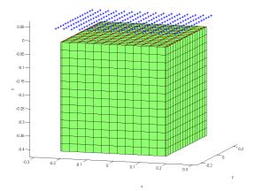
Figure 1: Sketch of the experimental setup. The box is shown with the BEM mesh used for the forward calculations. Measurement points for the vibrometer are indicated with red dots, and measurement points for the sound pressure are indicated with blue dots.
