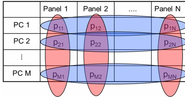
Figure 8 – For a specific principal component the panel contribution are added on vector basis (indicated by blue), while for a specific panel the contribution of the principal component, PC X are added on power basis (indicated by red)
