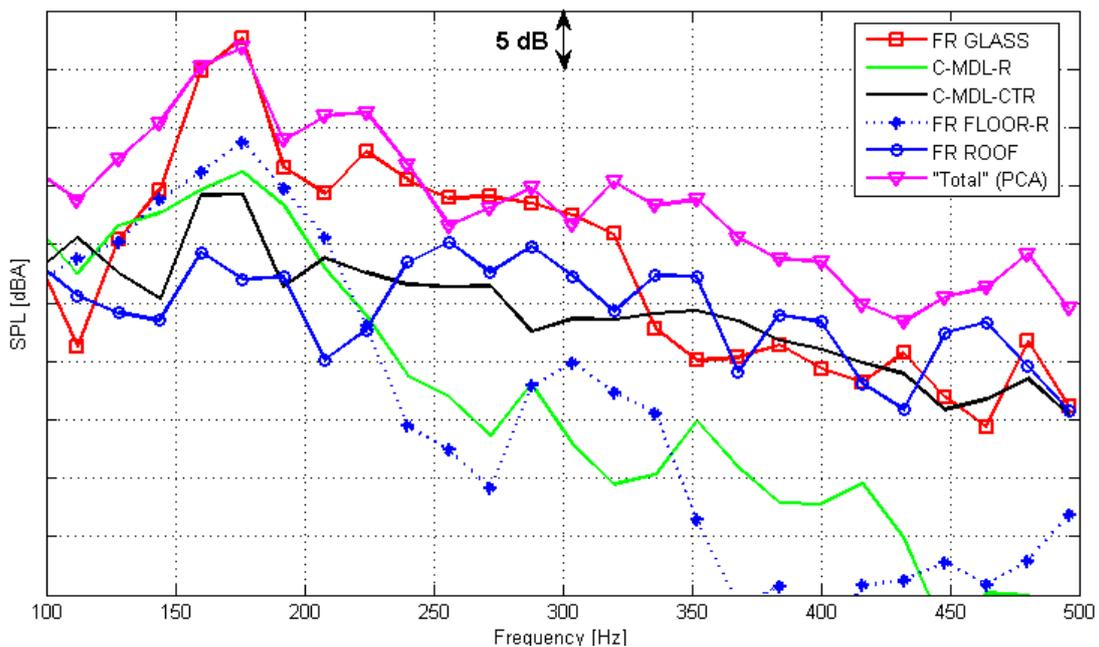
Figure 9 – Panel contribution analysis at driver’s position inside a passenger vehicle. Below 325Hz the wind shield (red curve) is the dominating contributor. Above 325 Hz the front roof (blue curve) becomes a significant contributor at several frequencies
