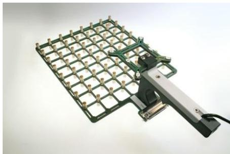
Figure 3a – Double layer array with 8x8x2 microphones
