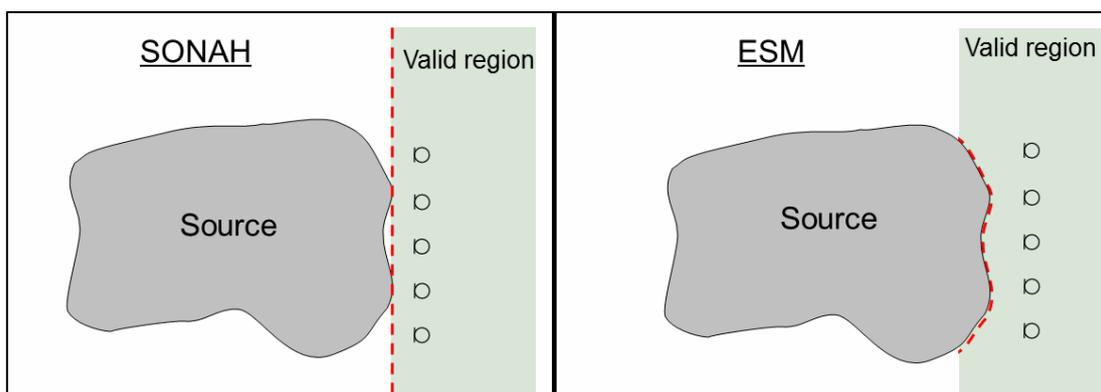
Figure 2a – Valid region of SONAH algorithm, Figure 2b – Valid region of ESM algorithm
