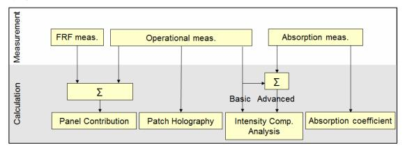
Figure 10 - Overview of the various measurement combinations for the four hand held array applications
