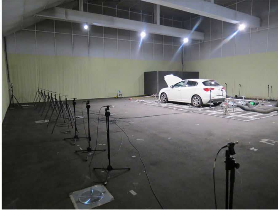
Figure 8: Single-side indoor pass-by measurement setup with additional indicator microphones for contribution analysis.
