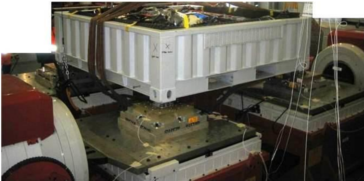
Figure A1 – Set up of horizontal test for 3 Ton 8 Foot Iso Container
