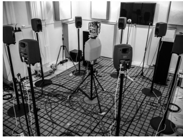
Figure 5: The loudspeaker setup in the IEC listening room
