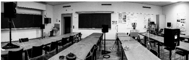
Figure 4: A reference background noise scene using 6 loudspeakers arbitrarily placed in a classroom.
