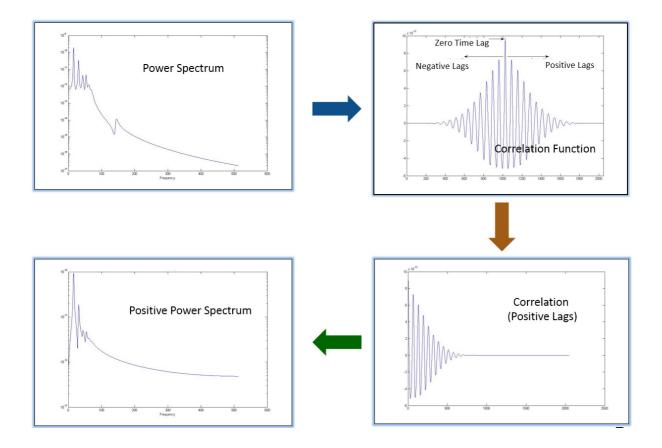
Figure 1. Calculation of Positive Power Spectrum.
