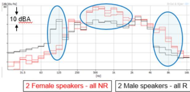
Figure 10. Spectral Difference between Female & Male Speakers for "Call Neal"
