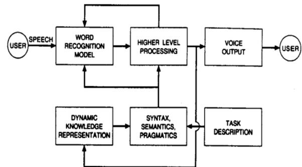
Figure 1. Block diagram of a task oriented voice recognition system
