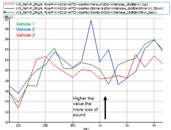
Figure 9. Transmission Loss from driver speech location to VR mic position
