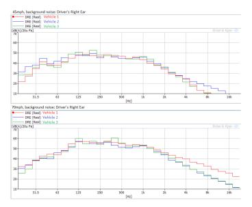
Figure 2. Background Noise Levels at 45mph (top) & 70mph (bottom)
