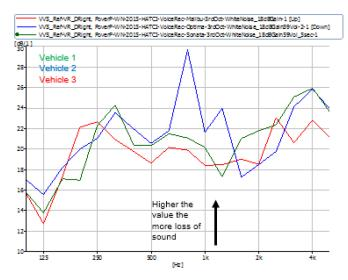
Figure 9. Transmission Loss from driver speech location to VR mic position
