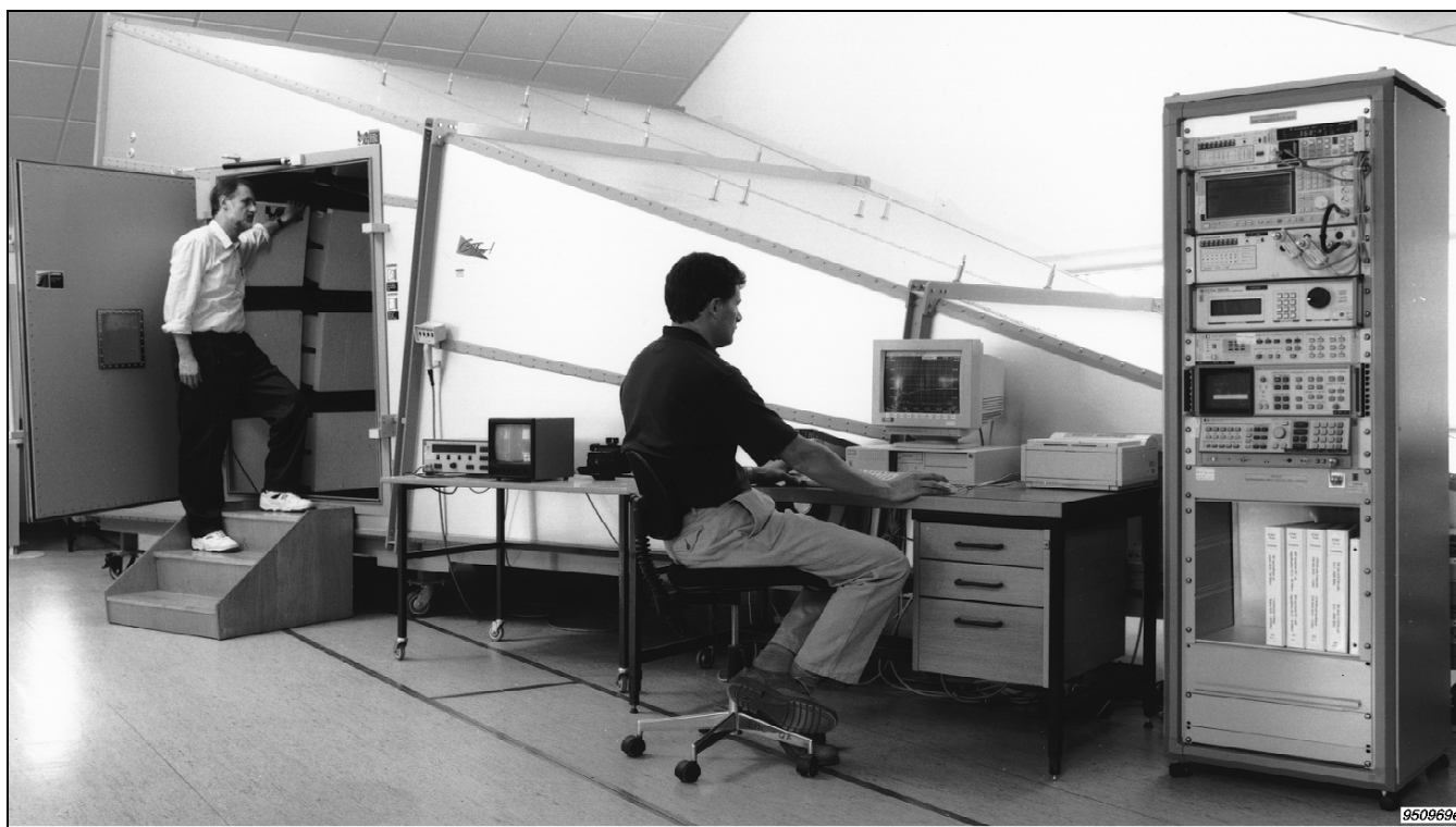
Fig 4.9 GTEM (Gigahertz Transversal Electromagnetic) test cell at Brüel & Kjær's EMC test laboratory: measuring radio frequency signals – emission and immunity
