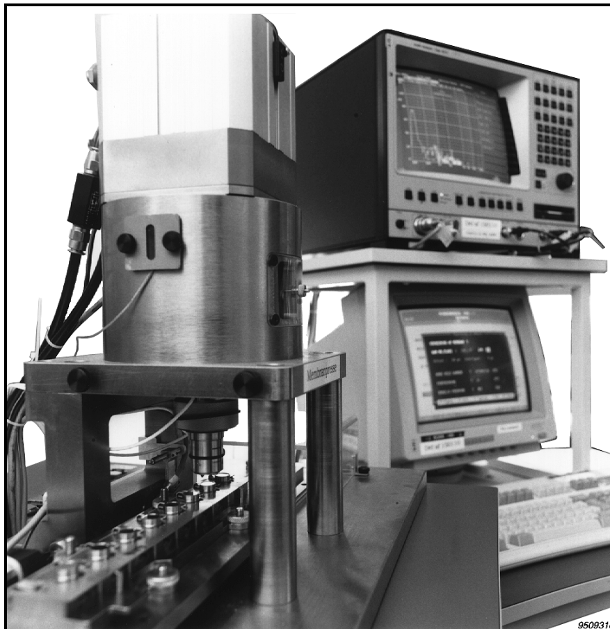
Fig. 1.8 Diaphragm press in use during production
