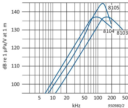
Hydrophone Types 8103, 8104 and 8105 can be used as sound transmitters (projectors), for both measurement and reciprocity calibration. Just as the piezoelectric effect produces an electrical output from mechanical excitation, applying alternating voltage to the transducer will produce mechanical excitation in the piezoelectric element.
