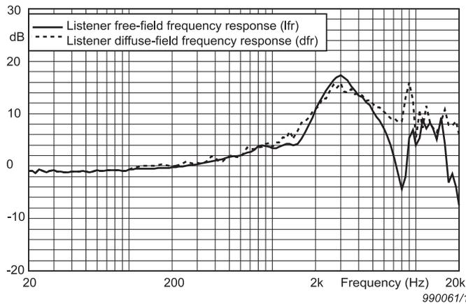
The combined influence of the torso, head, pinna and ear canal on airborne sound signals can be quantified by the acoustic free-field transfer function (the frequency response from free-field to the eardrum). This is called the listener free-field frequency response (lfr) or head related transfer function (HRTF) in telecommunications, and the manikin frequency response in technical audiology.
