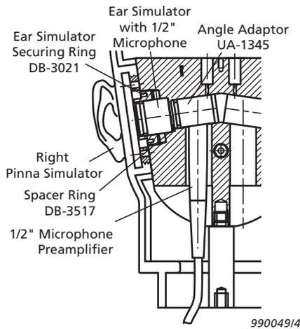
Each ear simulator consists of a removable silicon-rubber pinna joined to an ear canal. The ear canal ends in an occluded ear simulator that simulates the inner part of the ear canal according to the IEC 60318-4 standard. The ear simulator contains a 1/2" microphone and is connected to a microphone preamplifier with an adaptor. The ear simulator complies with ITU-T Rec. P.57 and ANSI S3.25.
