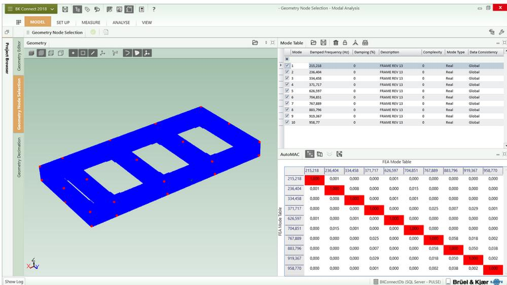
By logically grouping features and result displays, BK Connect Modal Analysis allows you to do a complete modal analysis in just four main steps:
