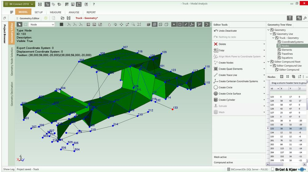
Finite element (FE) models can be imported and used in BK Connect Modal Analysis for pretest analysis and test validation.
