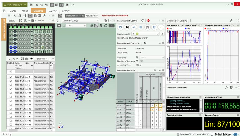
With BK Connect Modal Analysis, geometries can be created from scratch using the embedded drawing tools. You can work with various elements like points, lines, triangular or quad surfaces and you can create 2D and 3D CAD models and mesh them. The geometry can also be created from table entries.
