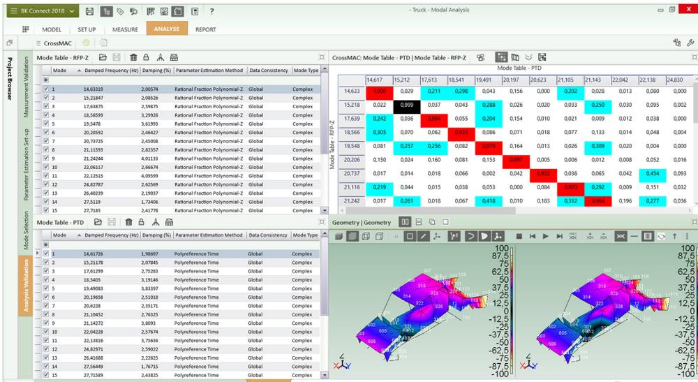
Fig. 9 Quad View colour contour animation of two mode shapes from a MSC Nastran FE model with more than 1 million nodes
