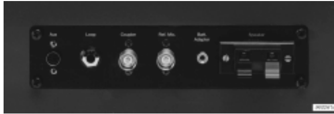
Fig. 2 Back panel of Anechoic Test Box Type 4232. All connections to the inside of the test box are made via the connectors on the back panel
