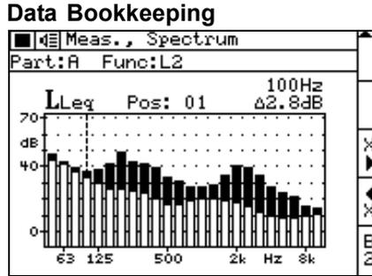
BZ-7204 has an automatic data bookkeeping system, that saves you the task of remembering file names, etc. It is a hierarchical system with a “Job” record at the top level. A Job is denoted by a four digit number. As an example, this could relate to a certain measurement location.
