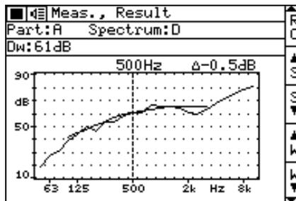
As soon as just one position of L1, L2, (B2) and T2 has been measured, the sound reduction index (spectrum and weighted) can be calculated. Generally the sound insulation is calculated (for each partition) from the average of all the positions of L1, L2, B2 and T2. It is possible to exclude positions from the average to see what effect certain positions have on the result. Several calculation formulae can be selected, depending on the selected standard.
