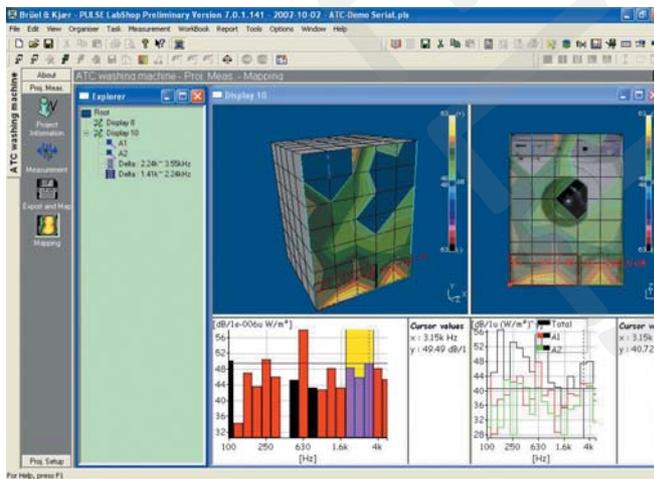
Once measurements have been made, result data can be displayed using the mapping software (see Fig. 3).
