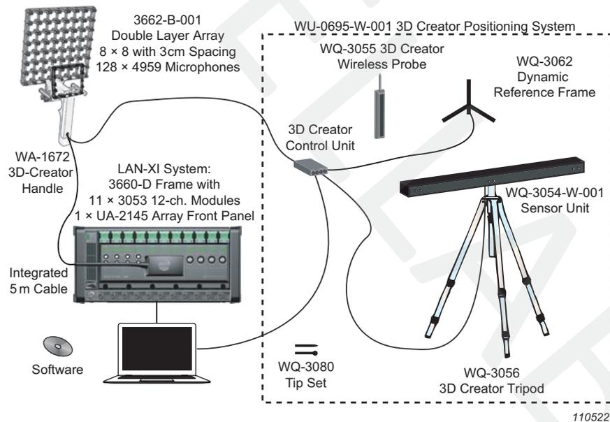
The array handle incorporates multiple infrared emitters that the sensor unit tracks and measures.
