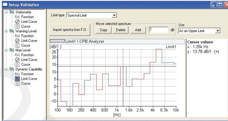
Validation ensures that measurements are reliable. It sets up the test criteria that are applied to measurement data and contains a Validation Tool which verifies that test data values follow standards or good measurement practice such as with dynamic capability, stationarity checks and other parameters. You can run validations against spectra, such as dynamic capability, to check for extraneous noise events, or
