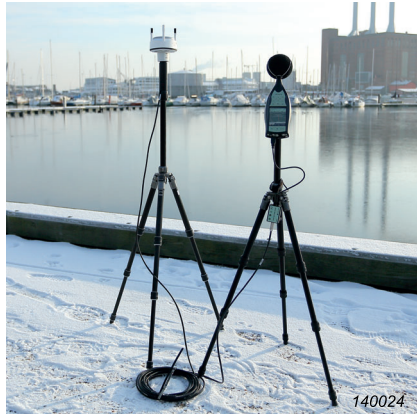
Fig. 13 Hand-held analyzer measuring outdoor noise using a weather station kit
