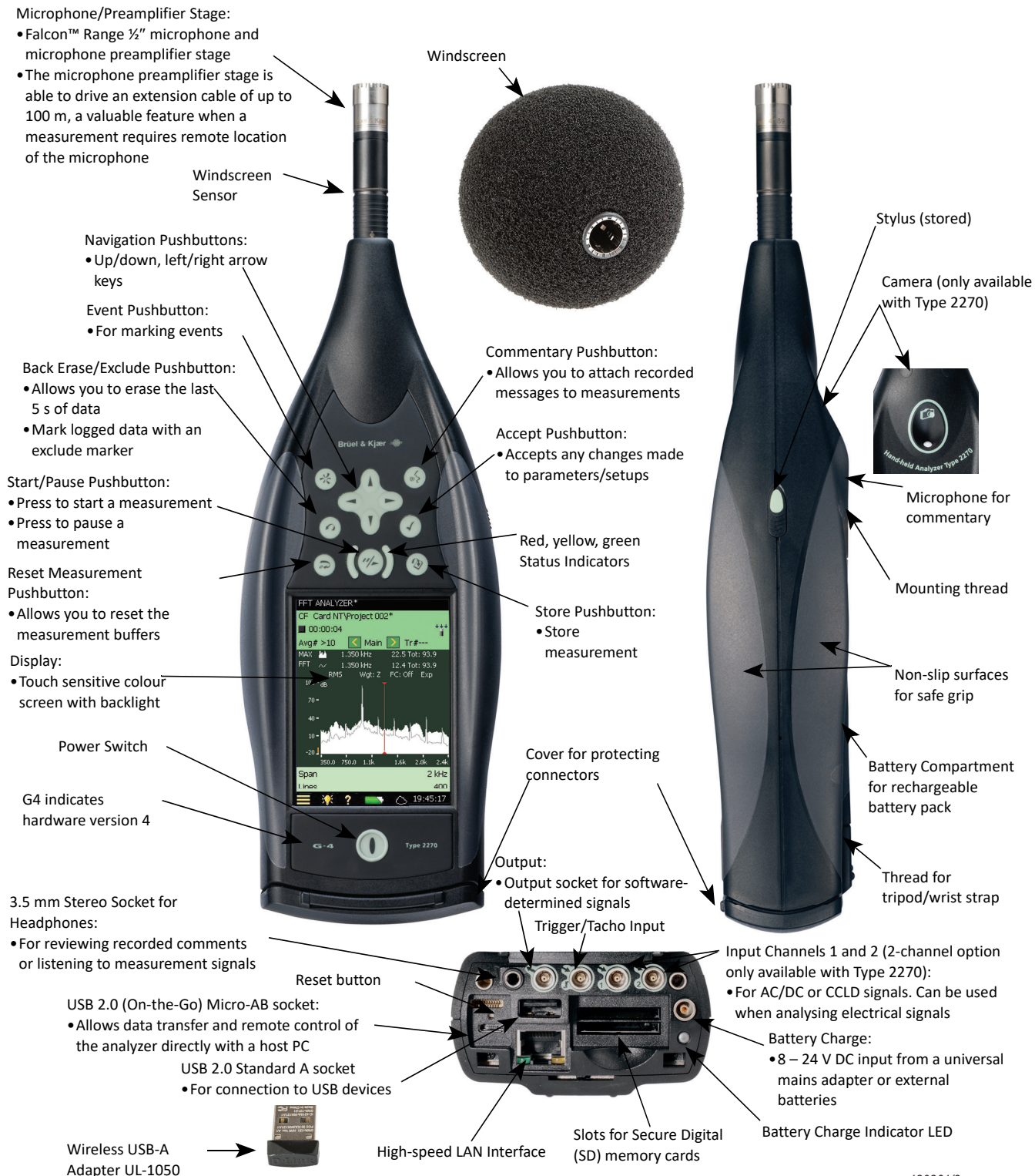
Fig. 1 Key features of Hand-held Analyzer Types 2250 and 2270
