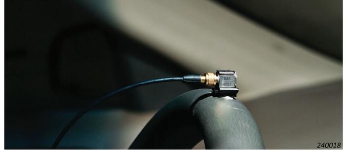
To shape and customize the mounting to fit your needs, use Mounting Clip with Thick Base UA-1475. The thick base can be filed down as needed.
