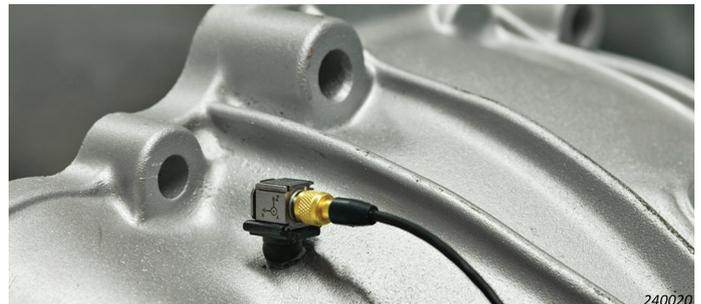
To align and realign the accelerometer without changing the coordinate system, use Swivel Base Clip UA-1478. Together with Spirit Level UA-1480, you can change the accelerometer's direction and still maintain the coordinate system.
