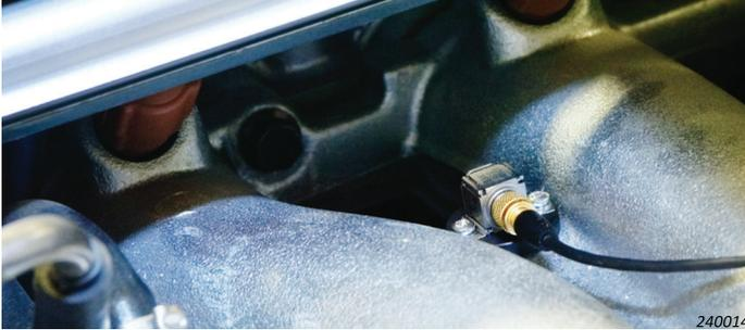
For mounting in high temperatures, use High-temperature Mounting Clip UA-1564.
