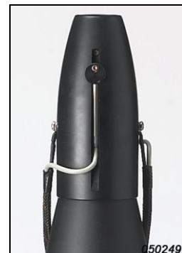
Fig. 1 Left: Top-view of Volume Velocity Adaptor showing phase-matched microphone arrangement. Right: Side-view of adaptor
