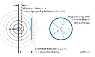
range: a low-frequency measurement at close range for SONAH and a high-frequency measurement at greater distance for beamforming. The patented Wideband Holography method can cover the combined frequency ranges of SONAH and beamforming based on a single measurement at an intermediate distance (Fig. 1).
