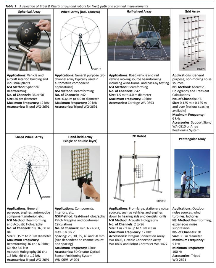
To improve overall noise levels, it is necessary to locate, quantify and rank the individual noise sources coming from a source. This starts by identifying 'hotspots' – areas where the local sound radiation is significantly greater than that of the surrounding area. Knowing these hotspots, the dominating frequencies and relative sound power contributions enable the cause of the noise to be identified and its contribution to the overall noise level to be assessed.
