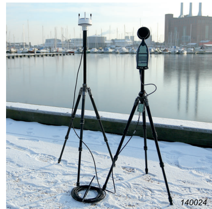
Fig. 6 Hand-held analyzer measuring outdoor noise using a weather station kit
