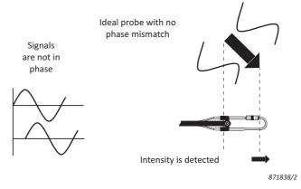
**Fig. 11** It is this apparent flow of acoustic energy that is detected and called "residual intensity"
