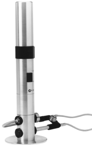
Fig. 4 Arrangement for sound intensity and particle velocity calibrations
