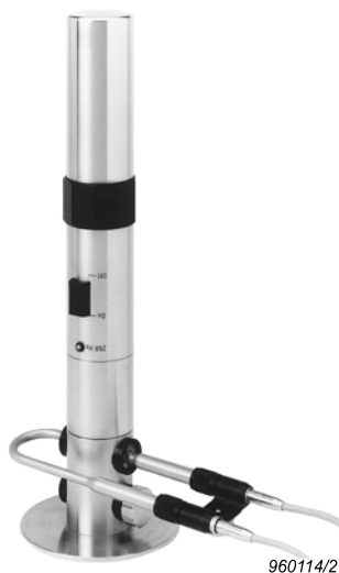
Fig. 2 Arrangement for sound pressure calibration. It can also be used to measure residual intensity and pressure-residual intensity index at 250 Hz
