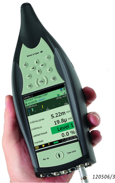
Fig. 1 The vibration analyzer (Engine Vibration Consultant). The simplified display shows only the required information, such as vibration level, limits and results
