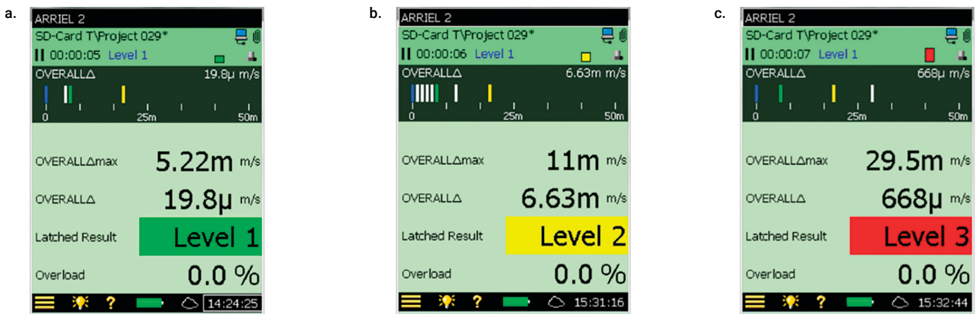
Fig. 5 Vibration check results on the acquisition page. a.: Green LEVEL 1: Keep the engine in service; b.: Yellow LEVEL 2: Unload and send the vibration raw data to SAFRAN HE for analysis. Refer to the engine maintenance manual for recommendations; c.: Red LEVEL 3: Unload and send the vibration raw data to SAFRAN HE for analysis. Refer to the engine maintenance manual for recommendations
