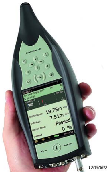
Fig. 1 Type 2250-H-100 Hand-held Vibration Analyzer (Engine Vibration Consultant) – the simplified display showing only the required information, such as vibration level, limits and pass/fail results
