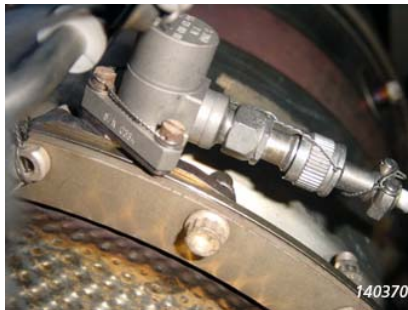
Fig. 3 Charge Accelerometer Type 8324 shown fitted to engine bracket
