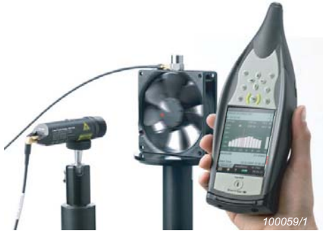
Fig. 1 Type 2981 with Hand-held FFT Analyzer Type 2250-H for product vibration testing
