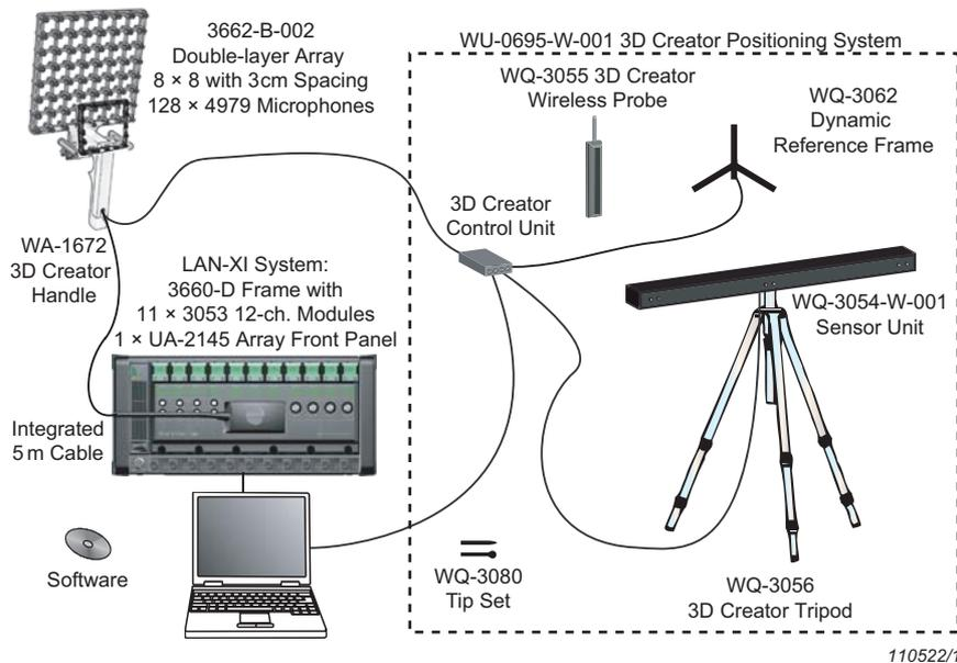
**Fig. 4** Acquisition system for panel contribution: double-layer hand-held array, PULSE LAN-XI front-end, 3D Creator Positioning System, volume velocity source, amplifier, generator and reference microphones
