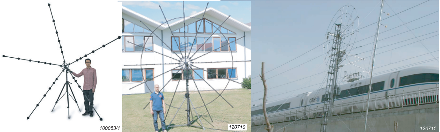
Fig. 1 Left: 30-channel pentangular array; Centre: 144-channel wheel array; Right: Example of an acoustic array used in measuring high-speed trains (photo courtesy of TPL, China)
