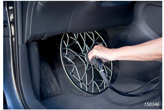
Fig. 4 Left: Hand-held Array WA-1764-W-001 with reflective plate for use in beamforming measurements Right: Without reflective plate for use in acoustic holography measurements
