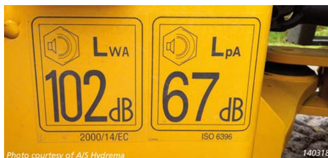
Fig. 2 Noise labels for sound power and pressure, A-weighted
