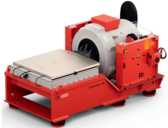
V8900 Combo-Mounted Shaker with HBT Slip Table
