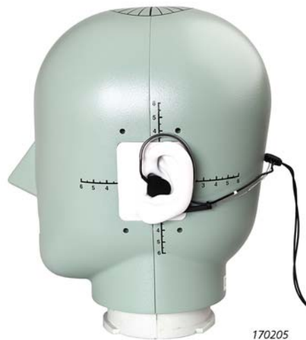
Fig. 1 Type 4101-B's microphone capsules rest in the concha of the ear, cushioned by foam windscreens. This makes for a comfortable fit inside a helmet
