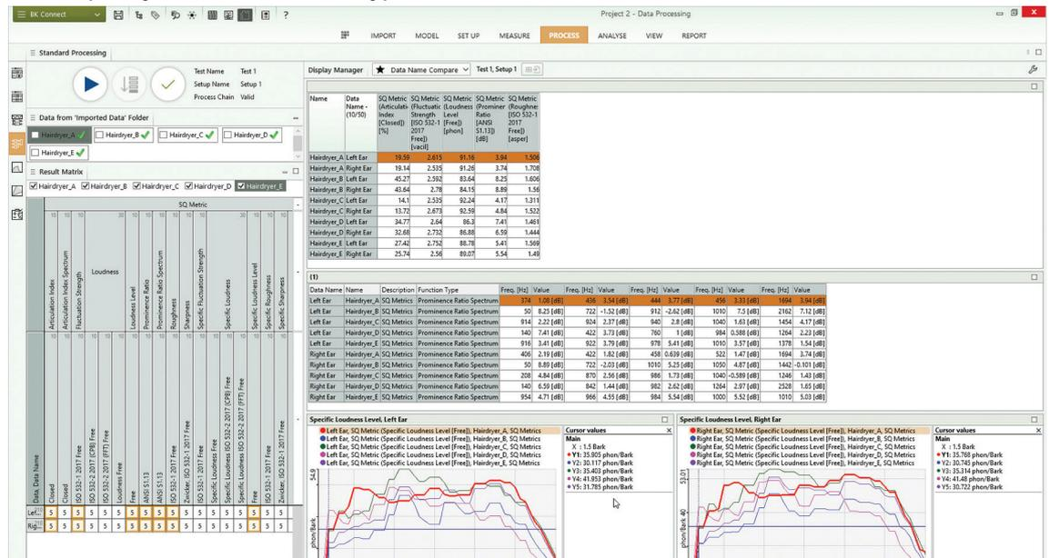
Type 8405-G adds sound quality metric calculations. Two specialized process chain elements enable the calculation of metrics as either overall values/spectra or as values/spectra versus time.
