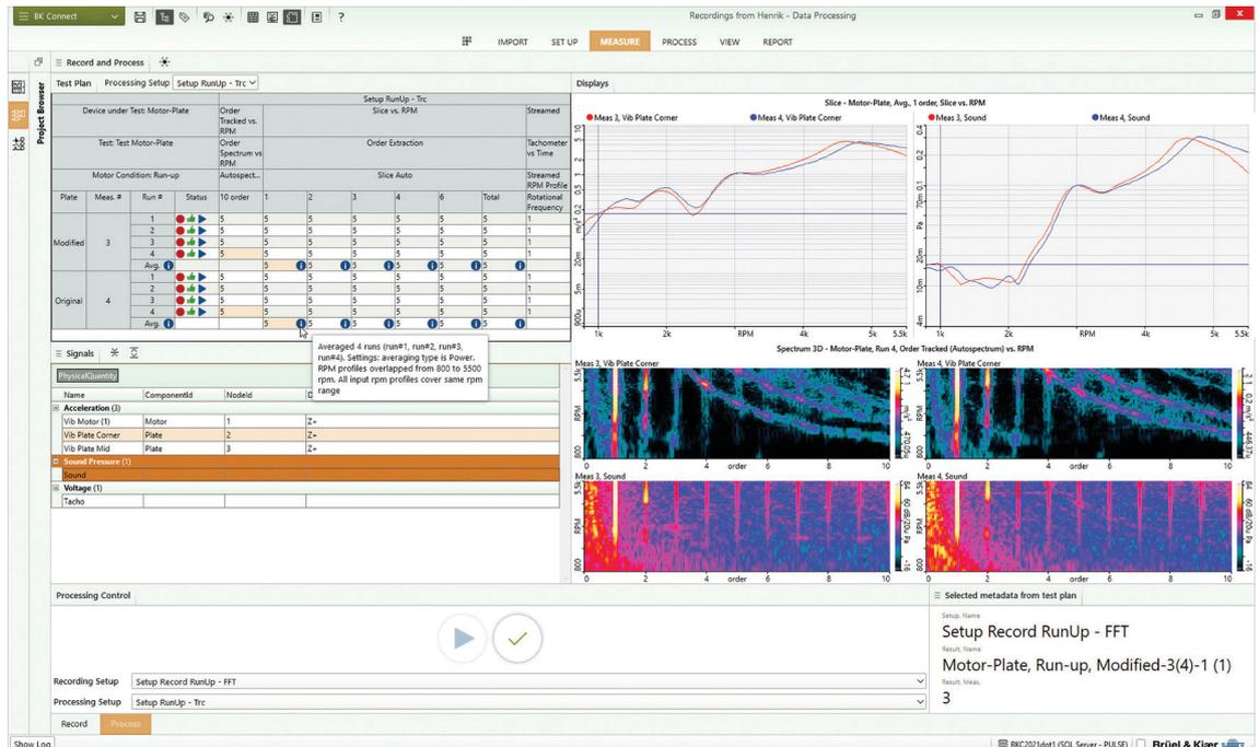
Type 8405-F adds tracked resampling to basic Type 8403/8403-A: Streamed data is resampled according to the instantaneous rpm value from a given tachometer signal.
