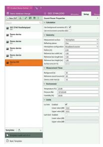
Perform Guided Measurements via Mobile Device or PC With a test or test template in hand, the test operator can then go step by step through a measurement using either the PC software or via a mobile device with the Product Noise Partner app downloaded.
