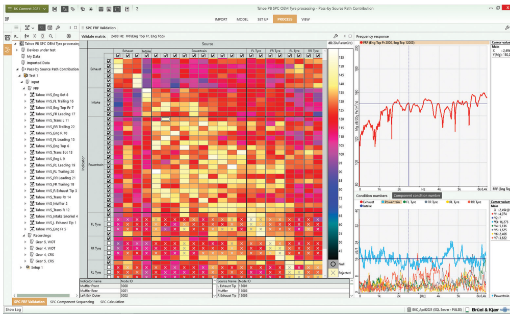
Fig. 4 The full matrix shown for a given frequency which is selected in the FRF graph
