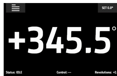
Fig. 1 Type 9640-A-001 touchscreen – displays the actual position of the turntable. Its also used to set up various turntable parameters via softkeys
