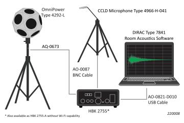
When HBK 2755 is connected to DIRAC over USB, the amplifier can be directly connected to a single CCLD microphone input, or up to two line-level inputs with external conditioning.
