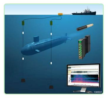
can be configured for specific needs covering the complete measurement chain from sensor (hydrophone) to analysis (PULSE™).
