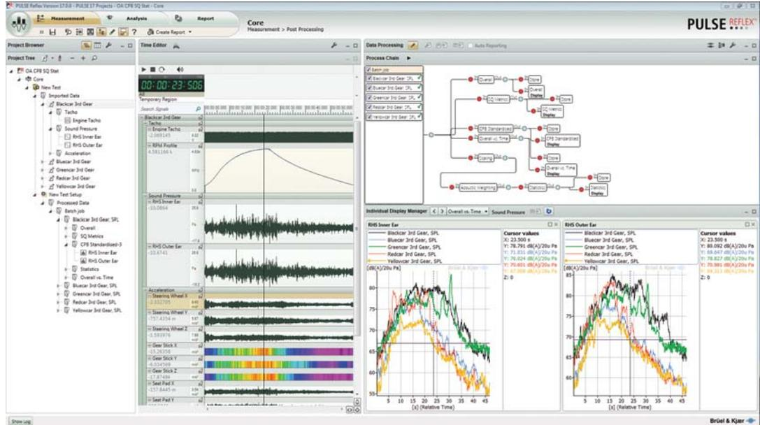
The tools are built into a framework that provides for fully automated operation, including batch processing for sequenced or parallel analysis of multiple sets of imported data.
