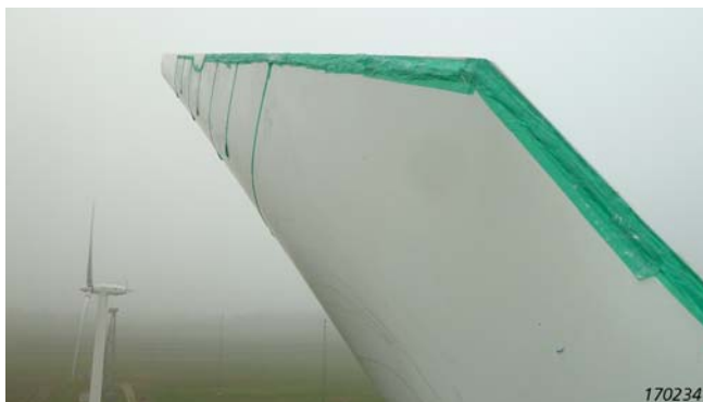
Fig. 6. Accelerometer cables running along the trailing edge of the blade
