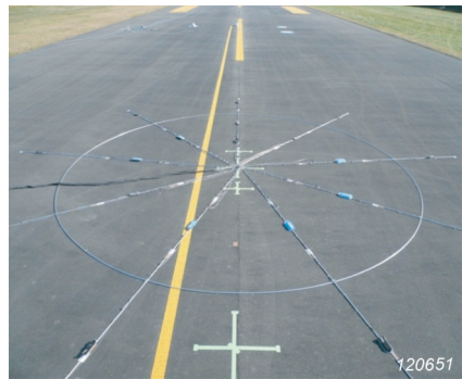
Fig. 1. Array geometry and picture of the array on the runway. Each microphone is clicked into position in the radial bars with the microphone tip touching the runway. "Half windscreens" can be added. The array diameter is 12 m, and there are 9 radial line arrays each with 12 microphones
