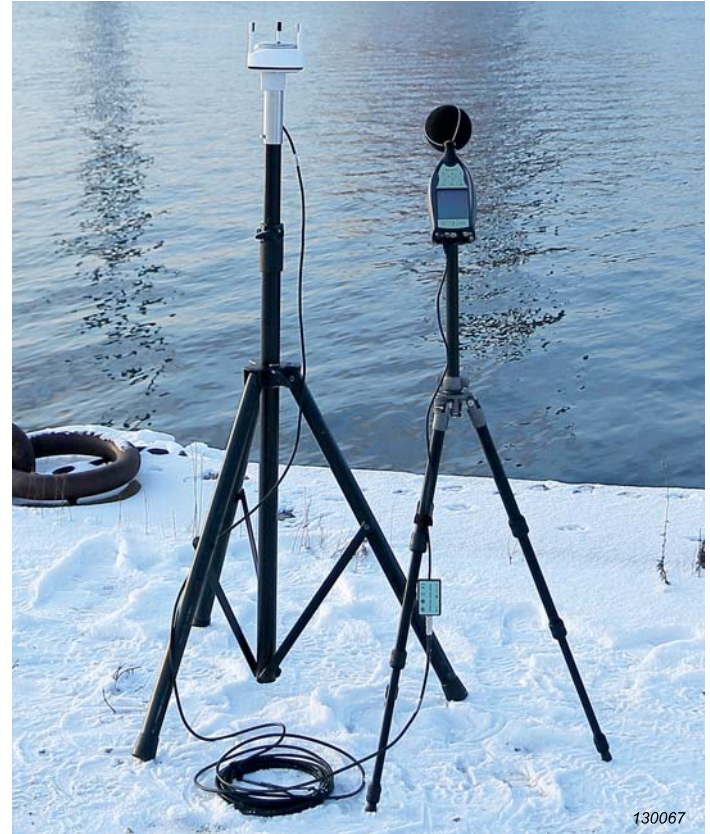
Configuration: Type 2250, weather station, speaker tripod and pole adaptor.
