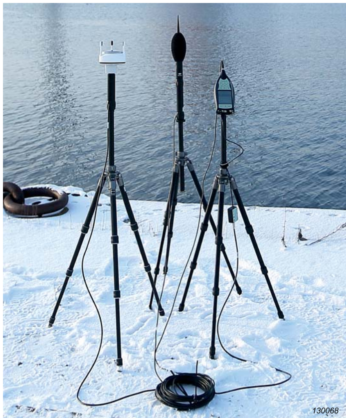
Configuration: Type 2250, weather station, Outdoor Microphone Type 4952, tripod and tripod adaptor
