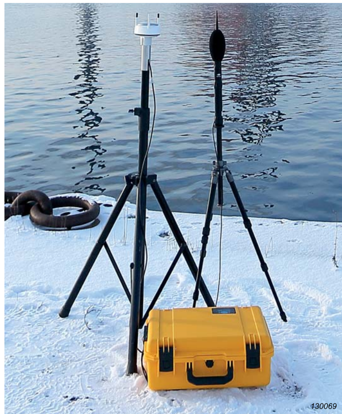
Configuration: Type 2250, weather station, ,All-weather Case Type 3535-A speaker tripod and pole adaptor
