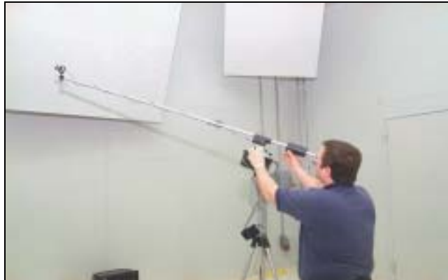
Fig. 6 David Copley adjusts a microphone inside the new reverberation chamber
