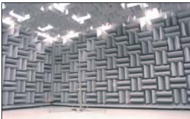
Fig. 4 An inside view of the hemi-anechoic chamber at Caterpillar's noise control research laboratory
