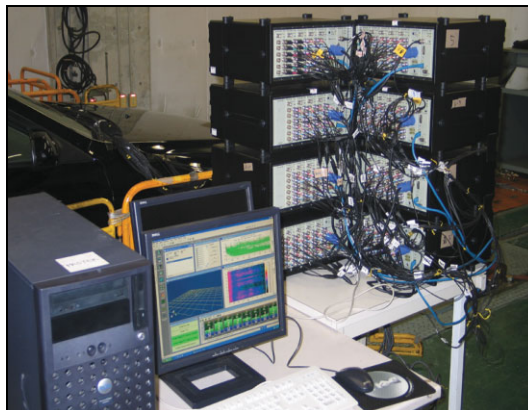
Fig. 1 Mazda ordered a large 220-channel PULSE system for modal analysis applications – the goal – to further optimise noise and vibration parameters in vehicle powertrains
