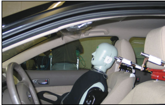
Fig. 4 A Brüel & Kjær Head and Torso Simulator Type 4128 C (HATS) is placed on the front passenger seat, and measures cabin noise on two channels – additional microphones are located in the cabin
